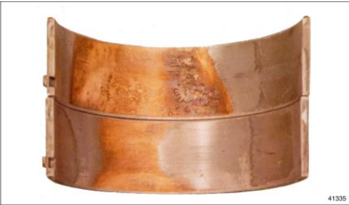
Figure 6-12 Example of Bearing Corrosion
