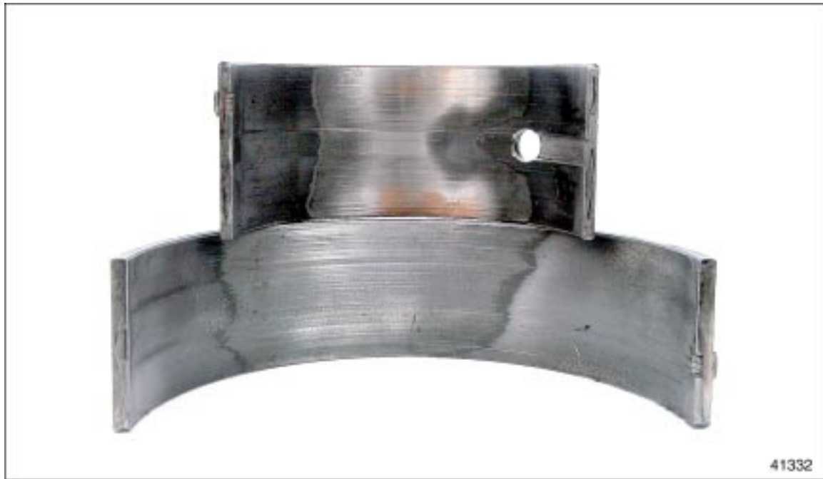
Figure 5-1 Bearing Wear under Normal Operation
