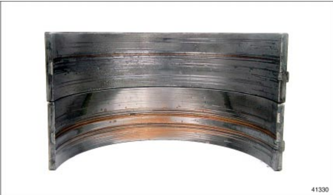
Figure 6-1 Example of Oil Contamination
