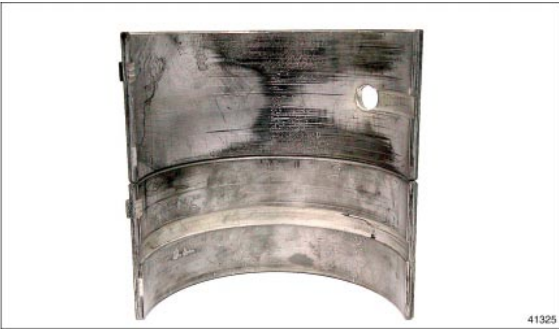
Figure 6-13 Example of Overlay Fatigue
