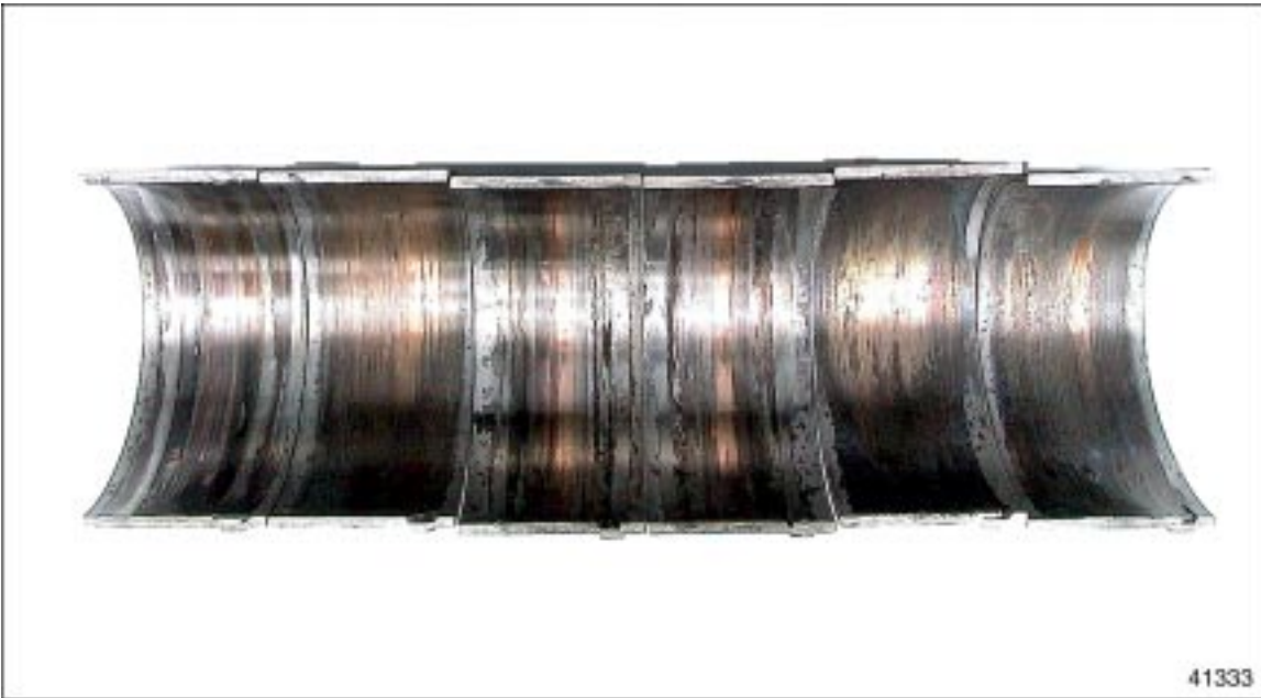
Figure 6-17 Example of Lack of Lubrication
