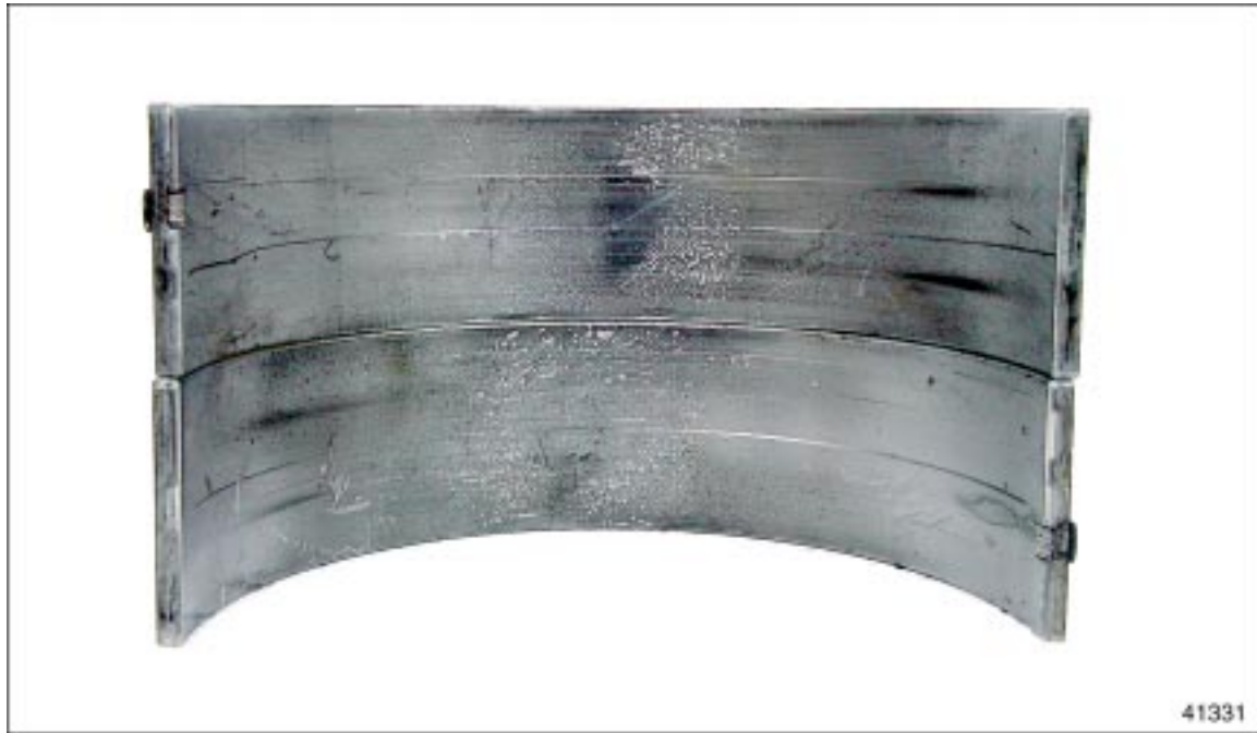
Figure 6-5 Example of Bearing Cavitation
