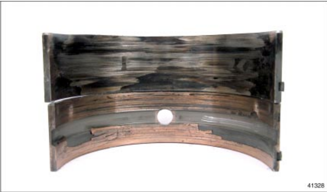
Figure 6-15 Example of Bearing Wiping
